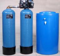
Duplex softeners are normally sized to give one regeneration per column per day, but each column can be regenerated more frequently if required. Parallel run systems with both vessels on line at the same time are also available.
